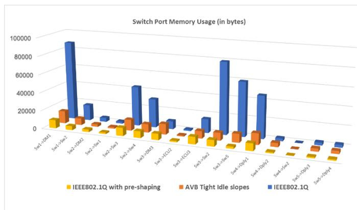
**Figure 7.** Upper bounds on the memory usage in the output ports of the switches with IEEE802.1Q (w/wo pre-shaping) and AVB Tight Idle slopes. The figures shown represent the sums for all the switches in the network.
