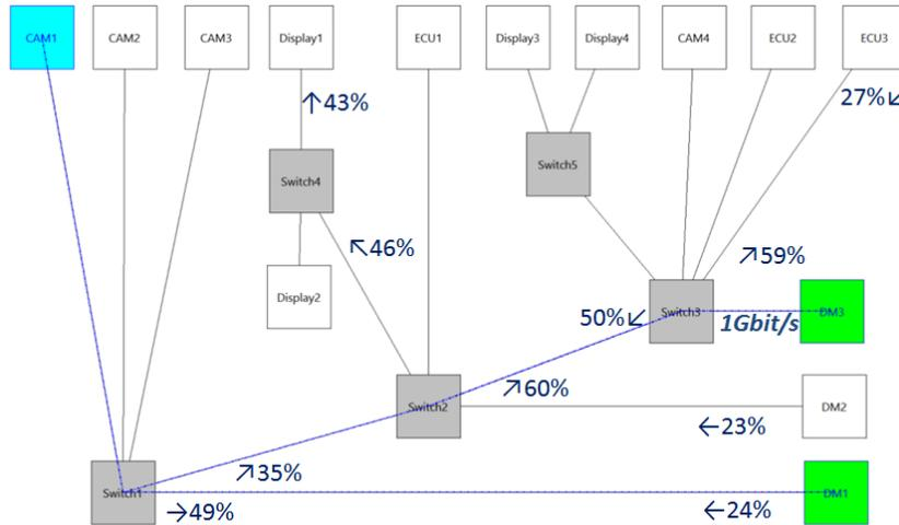
**Figure 2.** Topology of the prototype network used in the experiments. The multicast stream shown here goes from camera 1 to domain masters 1 and 3 (RTaW-Pegase screenshot). The graphic shows the 10 most loaded links, with a maximum of 60% load, and the single 1Gbit/s link. The traffic is made up of four classes for a total of 41 streams whose characteristics are summarized in Table 1.
