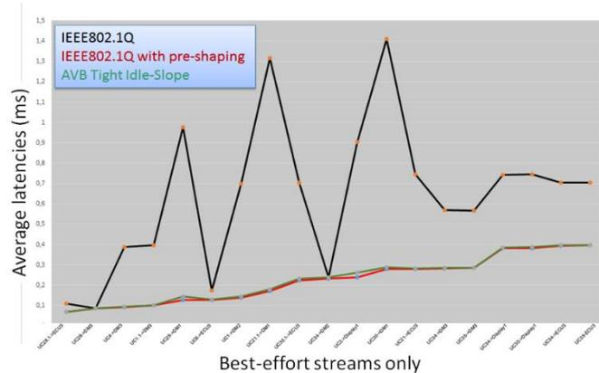
**Figure 4.** Average communication latencies for best effort under IEEE802.1Q, IEEE802.1Q with pre-shaping for video streams, and AVB/CBS configured with the tight idle-slope algorithm.
