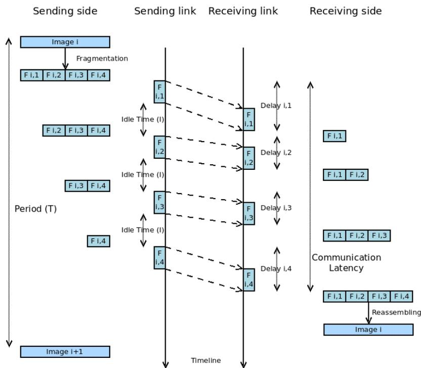
**Figure 1.** System model for the pre-shaping mechanism. A message, such as a camera frame, is transmitted with a period  $T$ . Each message is sent as  $N$  frames which are released for transmission each  $I$  time units. The last frame of the message will be released at time  $[N-1]I$  and must be received by the deadline.
