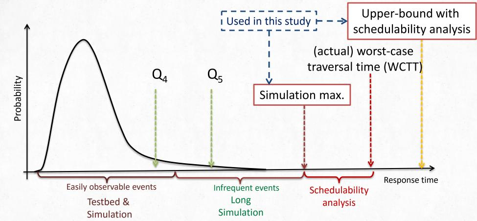
✓ Long simulation here = 48 hours of driving → 350 000 transmissions for 500ms frames
