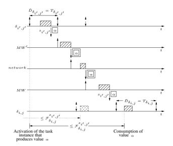
Figure 2. Scenario in which applicative task  $\delta_{i,j}$  consumes signal  $s_{i',j'}$  produced by applicative task  $\delta_{i',j'}$ . The configuration of applicative and middleware tasks and of the network frame must guarantee that the age of the values of  $s_{i',j'}$  respects the freshness constraint  $\mathcal{F}_{\delta_{i,j}}^{s_{i',j'}}$  associated to  $s_{i',j'}$ . Double square boxes represent a network frame that, in this case, carries value  $\alpha$ .
