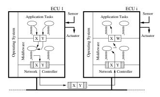
Figure 1. Part of an in-vehicle embedded system composed of two Electronic Control Units (ECUs) and a communication network. Each ECU contains a set of applicative tasks that periodically produce and consume signals through communication services provided by a middleware layer. This layer implements a mechanism that periodically packs and transmits signals into network frames.
