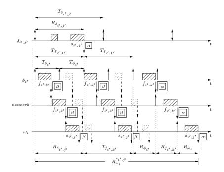
Figure 4. Scenario leading to the worst-case end-to-end response time  $R_{\omega_i}^{s_{i'},j'}$  of signal  $s_{i',j'}$ , from the activation of its producer task  $\delta_{i',j'}$  until the moment it is available for consumption in the receiver end. Shadowed boxes represent resp. the execution and the transmission of middleware tasks, resp. frames, that are not involved in the exchange of  $s_{i',j'}$ .
