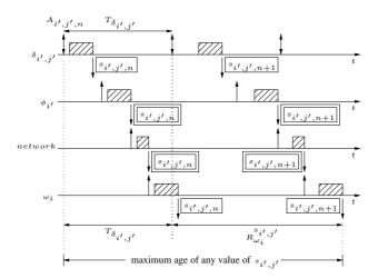
Figure 3. Illustration of the maximum age that the signal  $s_{i',j',n}$  can reach. Its age begins at  $A_{\delta_{i',j',n}}$ , the *n*-th activation of its producer task. In the worst case, the next instance of the signal,  $s_{i',j',n+1}$ , is available  $T_{\delta_{i',j'}} + R_{\omega_i}^{s_{i',j'}}$  units of time later. The maximum age that any signal  $s_{i',j'}$  can reach is  $T_{\delta_{i',j'}} + R_{\omega_i}^{s_{i',j'}}$ . Double square boxes represent a network frame.
