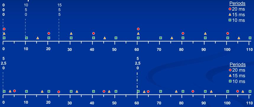
Algorithms to decide offsets are based on arithmetical properties of the periods and size of the frame
