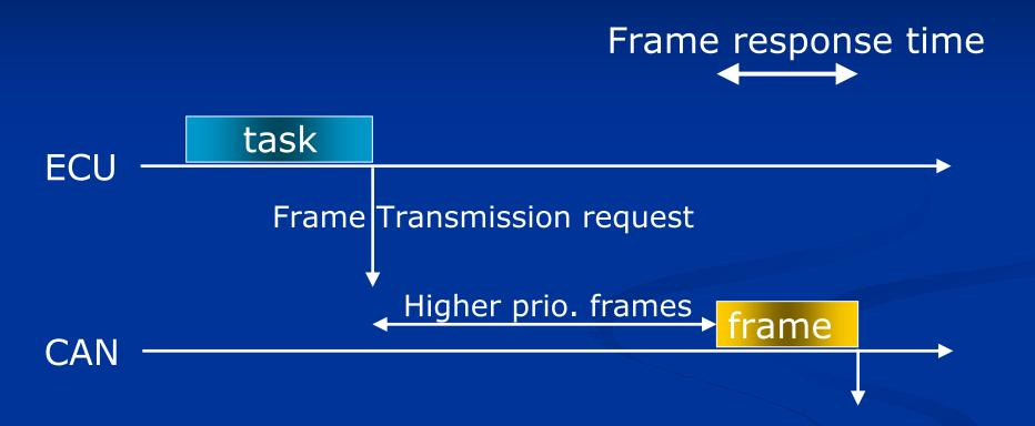
In addition, avoiding consecutive frame constructions on an ECU allows to reduce latency
