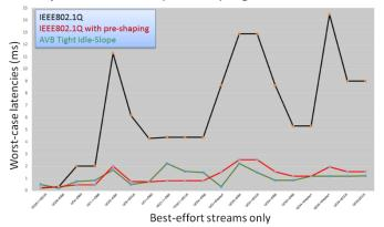
**Figure 5.** Worst-case communication latencies for best effort under IEEE802.1Q, IEEE802.1Q with pre-shaping for video streams, and AVB configured with the tight idle slope mechanism.
