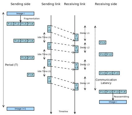
**Figure 1.** System model for the pre-shaping mechanism. A message, such as a camera frame, is transmitted with a period T. Each message is sent as N frames which are released for transmission each / time units. The last frame of the message will be released at time (N-1)·/ and must be received by the deadline.
