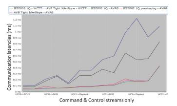
**Figure 6.** Worst-case and average communication latencies for Command and Control streams under IEEE802.1Q, IEEE802.1Q with pre-shaping for video streams, and AVB/CBS for Audio/Video configured with the tight idle-slope algorithm. The worst-case latencies for IEEE802.1Q with pre-shaping are all strictly equal to the ones obtained with pre-shaping.
