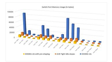
**Figure 7.** Upper bounds on the memory usage in the output ports of the switches with IEEE802.1Q (w/wo pre-shaping) and AVB Tight Idle slopes. The figures shown represent the sums for all the switches in the network.
