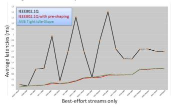
**Figure 4.** Average communication latencies for best effort under IEEE802.1Q, IEEE802.1Q with pre-shaping for video streams, and AVB/CBS configured with the tight idle-slope algorithm.
